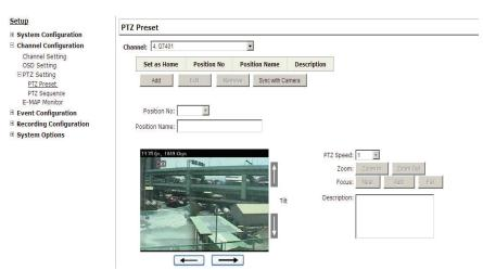
1. To set up PTZ preset points, select a camera from the "Camera" drop-down menu and click "Add"
