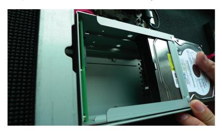
Make sure the SATA connectors are aligned with each other correctly
