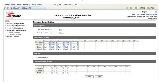
The "recording configurations" gives users the overall control of how and when a recording is performed and the quality of different types of recordings performed on each channels. It can help the recorder to operate with sufficient system resource by performing recording only when it's necessary with adjustable recording frame rate.
