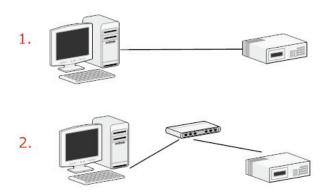
The PC that is connected directly to the NVR (or within the same local area network) should receive an IP from it. Simply access the NVR from your web browser with its IP address
