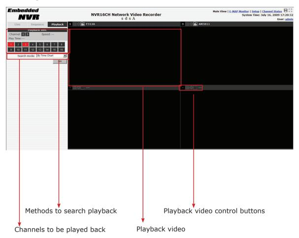
Playback is a function that allows you to play one or more videos that were previously recorded by a chosen recording method or due to an event trigger. The NVR offers synchronized playback from up to 4 channels and various types of search methods are provided to help you find the footage you need quickly.
