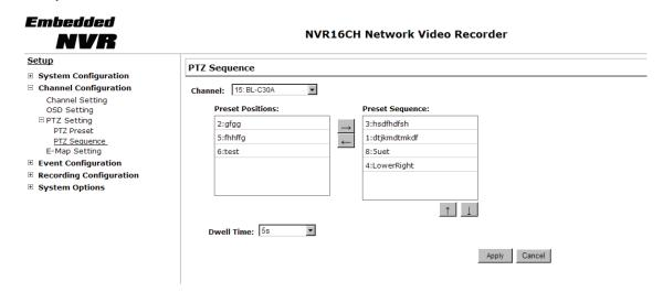
To configure preset sequence for a camera," select a camera from the "Camera" drop-down menu
