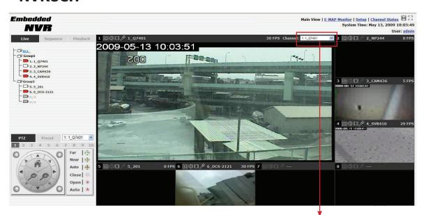
The 8 channel NVR comes with a 8-video split window view with one video displays on a larger window. Select a channel from the drop-down menu to display its video on the larger split window. You can also double-click on any of the smaller one to display its video to the larger window.
