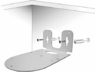
2. Fix the camera to L-type bracket with the two supplied screws
