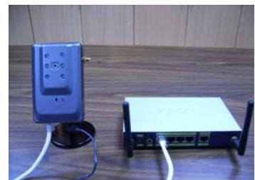
LAN port located on the Network Camera's bottom and attach the other end to the network device (hub or switch).
