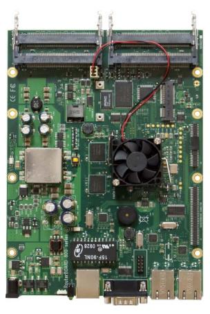
The RB800 is an advanced high performance wireless platform. It has four miniPCI slots, three Gigabit ethernet ports, two daughterboard connectors, a miniPCI-e slot and a compact flash slot. The two daughterboard connectors allow you to expand the number of wired and wireless ports, and the new high power CPU is capable of supporting them all.
